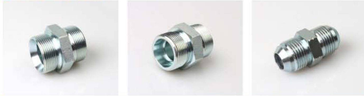
PART NO:1B BSP male double use for 60° seat or bonded seal PART NO:1C/1D Metric Male 24° Cone Seat L.T./H.T. PART NO:1J JIC male 74° cone
