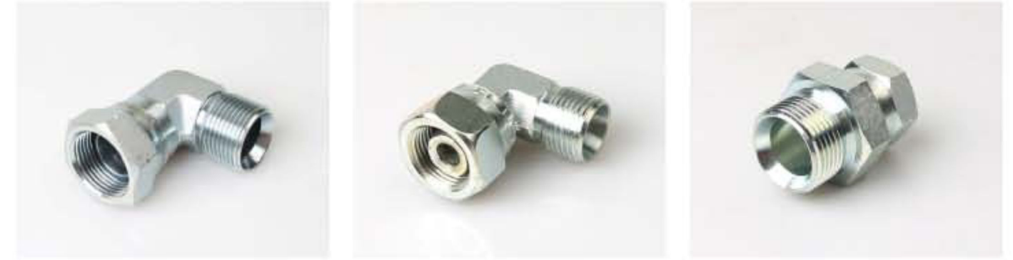
PART NO:2B9 90° elbow BSP male 60° seat/BSPT female 60° cone PART NO:2C9 90° elbow reducer tube adapter with swivel nut PART NO:2B BSP male double use for 60° seat or bonded seal/BSPT female 60° cone
