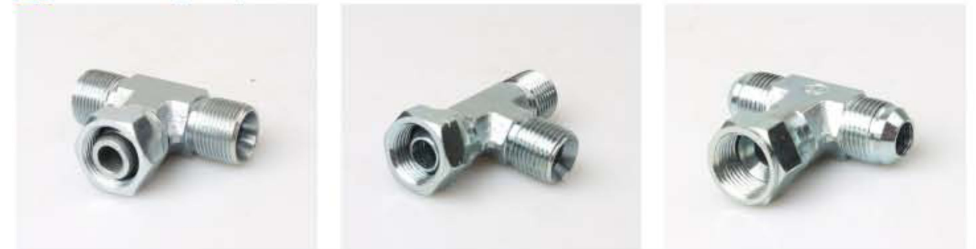
PART NO:BC Branch Tee Fittings With Swivel Nut PART NO:CB BSP Male 60° Seat/BSP Female 60° Cone Run Tee PART NO:BJ JIC male 74° Cone/ JIC Female Branch Tee
