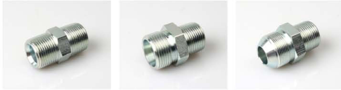
PART NO:1T BSPT Male PART NO:1CT Metric Male 24° Cone Seat/BSPT Male PART NO:1JT JIC male 74° Cone/BSPT Male
