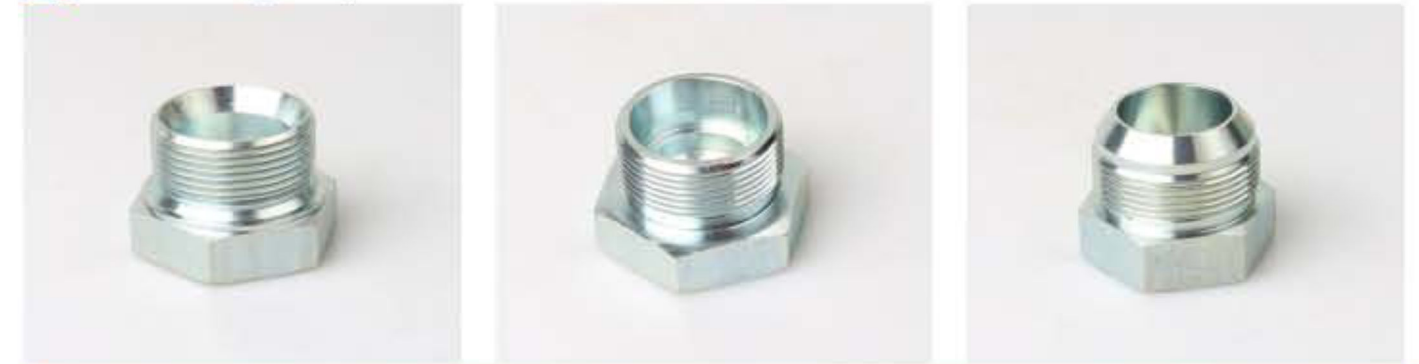
PART NO:4B BSP male double use for 60° seat or bonded seal plug PART NO:4C Metric Male 24° Cone Seat Plug PART NO:4J JIC male 74° cone plug
